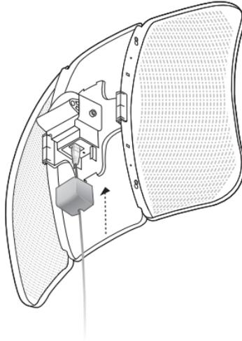
5. Attach the Mounting Bracket to the Rear Cover until the grooves on the Mounting Bracket are positioned over the pins on the Rear Cover.
