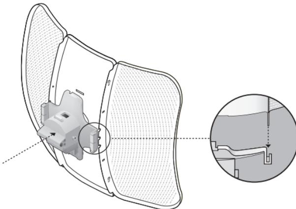
b. Attach the Rear Cover to the reflector assembly. Press upon the Rear Cover at the four positions marked in the diagram below in sequence until it locks into place.
