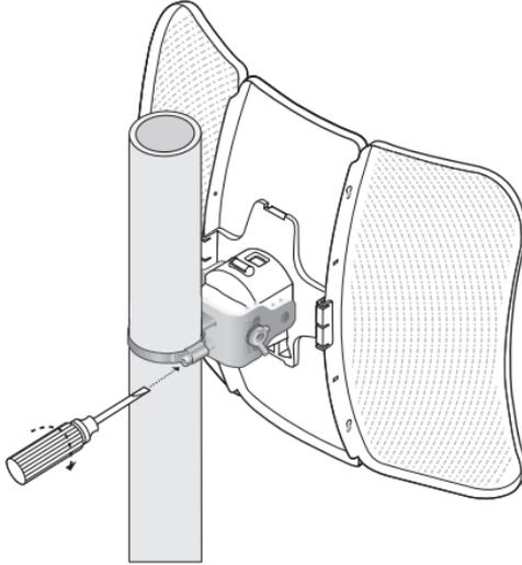
8. Adjust the azimuth and elevation angle of the CPE device to achieve maximum signal strength.
