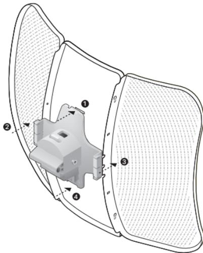
**WARNING:** To avoid damage, do not place the panels on a flat surface or push down on it.
