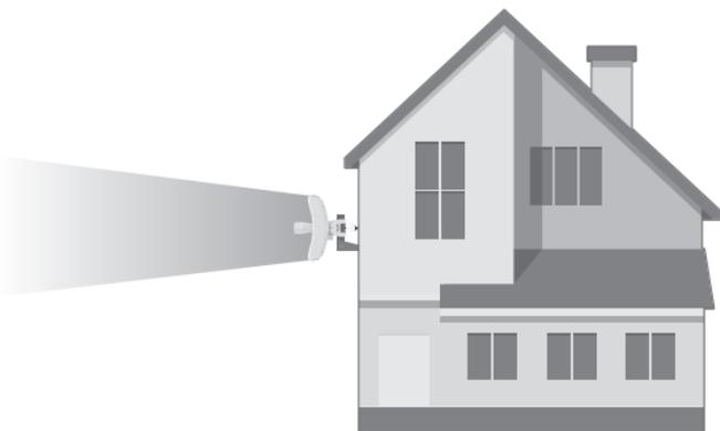
The CPE device without the reflector installed provides outdoor-to-indoor Wi-Fi coverage with the Feed only mode.
