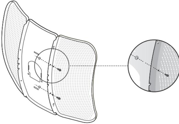
2. Attach the Rear Cover to the reflector assembly as follows:
