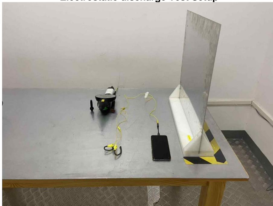
Electrostatic discharge Test Setup
