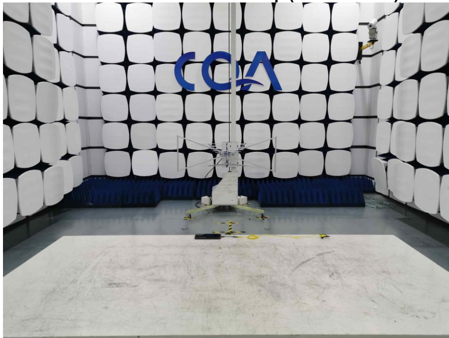
Radiated emission Test Setup (30MHz~1GHz)
