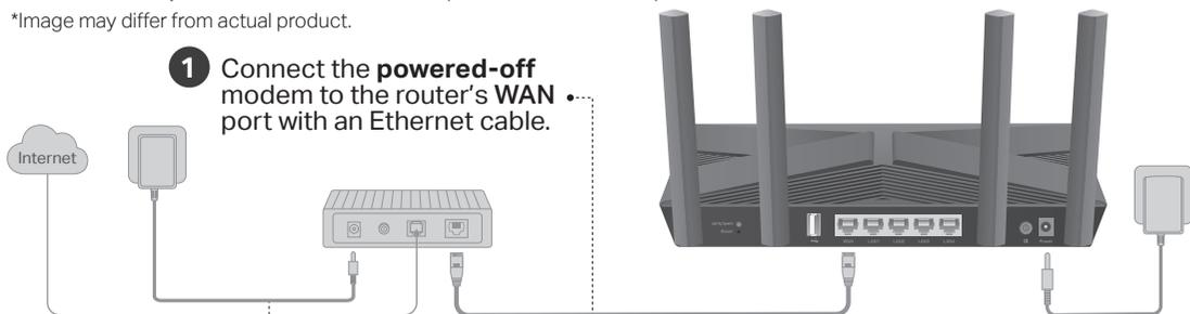
**1** Connect the **powered-off** modem to the router's **WAN port** with an Ethernet cable.
