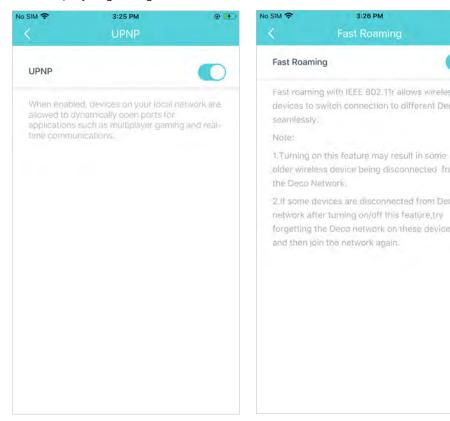
Enable Fast Roaming to allow your wireless devices to switch connection to different Decos
