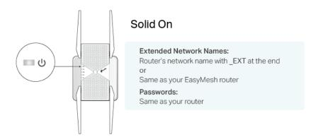
If you cannot find the network names with **\_EXT** in your Wi-Fi network list, this means that the extender has been connected to a EasyMesh router and automatically copied its wireless settings.
