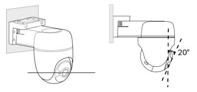
5. Mount your camera to the side so that movement goes across the lens' field of view to better trigger motion detection and Al detection.
