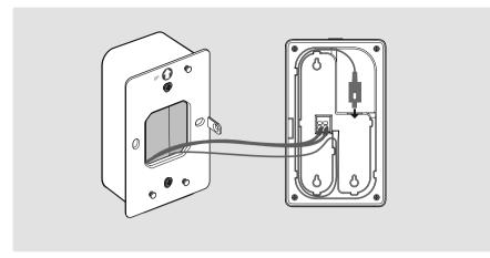
5. Attach the EAP to the mounting bracket. Secure them with the provided screw.
