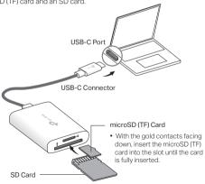
With the gold contacts facing up, insert the SD card into the slot until the card is fully inserted.
