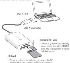
card into the slot until the card is fully inserted.
