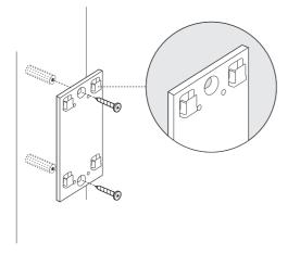
2. Attach the passive PoE adapter to the mounting bracket by sliding the adapter in the direction of the arrows until it locks into place.
