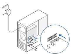
d. Locate an available F\_USB connector and carefully plug the Bluetooth USB cable into it.
