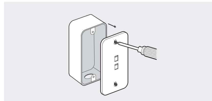
2. Secure the mounting bracket to the junction box with the provided screws.
