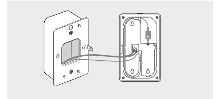
5. Attach the EAP to the mounting bracket. Secure them with the provided screw.
