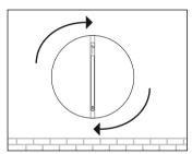
Attach the Festa AP to the mounting bracket by rotating it until it locks into place, as shown on the left.
