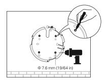
If your Ethernet cable feeds through the wall, position the mounting bracket below the cable hole. Mark positions for the screw holes and drill holes at the marked positions.
