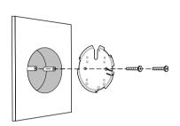
Route the cables through the square cable hole on the mounting bracket, and secure the mounting bracket to the junction box using screws
