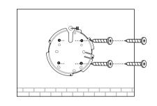
Secure the mounting bracket to the wall by driving the self-tapping screws into the anchors. Make sure that the shoulders of the mounting bracket are on the outside.
