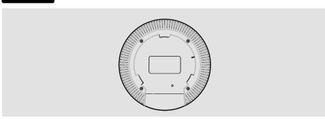
With the device powered on, press and hold the button for about 5 seconds until the LED flashes quickly. Then release the button. The device will restore to factory default settings.
