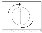
Attach the Festa AP to the mounting bracket by rotating it until it locks into place, as shown on the left.
