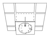
Feed the Ethernet cable through the hole and set the ceiling tile back into place.
