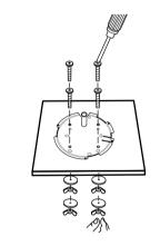
3 Secure the mounting bracket to the ceiling tile using pan-head screws, washers, and wing nuts, as shown on the left.
