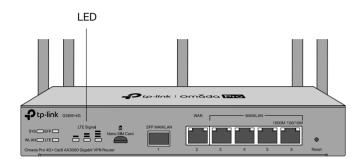
Reset: Press and hold the button for 5 seconds, the SYS LED will flash quickly, indicating the device is being reset to its factory default settings.
