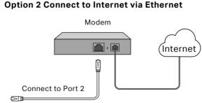
Note: To connect to the internet via another RJ45 WAN port (ports 3-6), configure your desired port to WAN, then connect the port to the internet via an RJ45 cable. Refer to FAQ-Q1 for more details.
