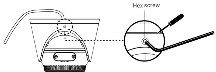
**Option 2: Route the cable through the side outlet.** Insert anchors into the holes and use screws to affix the camera base. Identify the groove and alignment ridge on the camera. Begin by aligning the base's rim with the camera's groove, attaching the ridge side first for a correct fit. Once aligned, proceed to snap the rest of the camera onto the base to secure it.
