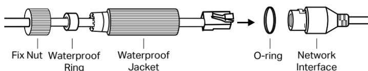
1. Route the network cable through the following components in order: fix nut, waterproof ring, and then the waterproof jacket.
